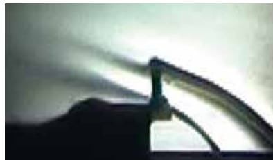
Cross section through sash and side post. Due to the special design, ambient air is flowing in like being accelerated through a nozzle without jeopardising the splash protection.
